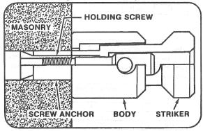
Screw Anchor Expanders--Hardened alloy steel.
